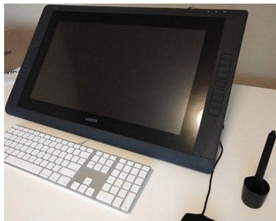
Fig 2. Multi-touch and pen-input capable monitor with mouse and keyboard
